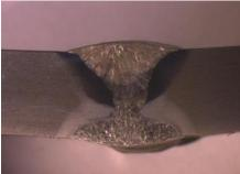
Figure.1.Macro examination of the specimen revealed complete weld fusion
